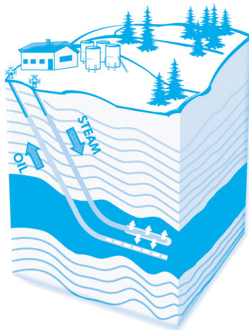
FIGURE 7: Steam Assisted Gravity Drainage Process (SAGD Process)
